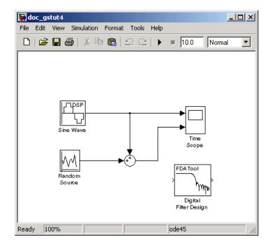
**2** Incorporate the Digital Filter Design block into your block diagram. Click-and-drag the Digital Filter Design block, and place it between the Random Source block and the Sum block.
