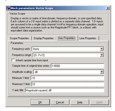
After you have set the block parameter values, you can calculate and view the power spectrum of the speech signal. To learn how to do this, see "Viewing the Power Spectrum Estimates" on page 6-8.
