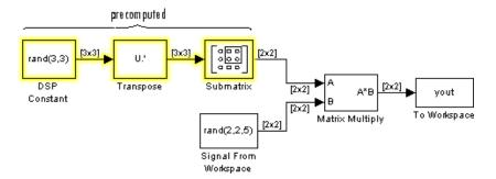
This process eliminates the computational overhead of continuously reevaluating these constant branches, which results in faster simulation and smaller, more efficient generated code.
