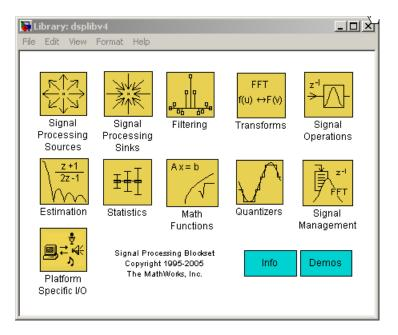
2 Double-click the Signal Processing Sources library. The library displays the blocks it contains. The orange blocks support fixed-point data types in some or all modes. You can use the blocks in the Signal Processing Sources library to create discrete-time or continuous-time signals.
