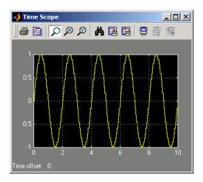
You can achieve a more finely sampled output by decreasing the **Sample time** parameter. For example, change the **Sample time** parameter to 0.005, run the model, and autoscale the output. The **Time Scope** window should now look similar to the following figure.
