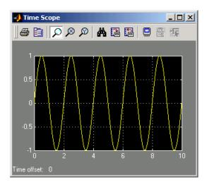
**5** Experiment with your model. Change the **Frequency** (**Hz**) and **Sample time** parameters of the Sine Wave block. Then, run your model to see the effect.
