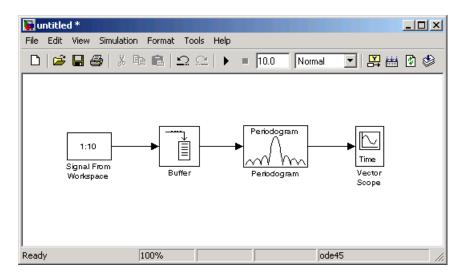
Once you have assembled the blocks needed to calculate the power spectrum of your speech signal, you can set the block parameters. To learn how to do this, see "Setting the Model Parameters" on page 6-3. The Buffer, Periodogram, and Vector Scope blocks in this model can be replaced by a Spectrum Scope block. For more information on this block, see the Spectrum Scope block reference page.
