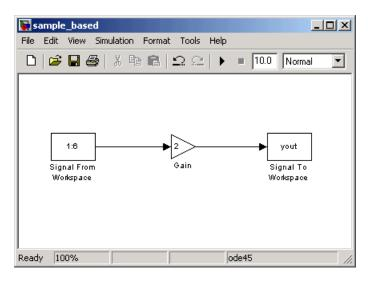
The Signal From Workspace block outputs a sample-based signal. The Gain block multiplies all the samples of the signal by two. Then, the Signal To Workspace block outputs the signal to the MATLAB workspace in the form of a variable called yout. The following figure is a symbolic representation of how the single-channel, sample-based signal is propagated through the model.
