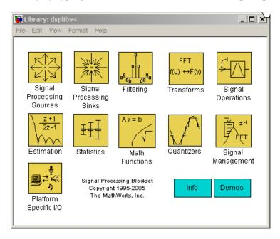
**2** Open a new model. In the Signal Processing Blockset library window, click on the **File** menu, point to **New**, and select **Model**. You can drag-and-drop Simulink blocks into a model to represent a system and model its behavior.
