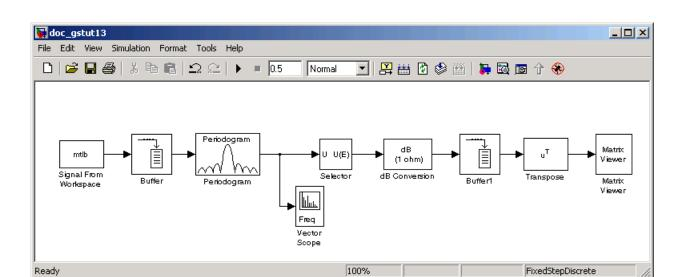
**2** Run the model. During the simulation, the **Vector Scope** window displays a sequence of power spectrums, one for each window of the original speech signal. The power spectrum is the contribution of every frequency to the power of the speech signal.
