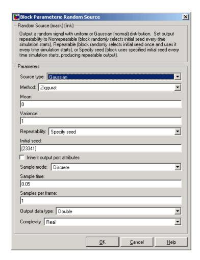
Opening this dialog box causes a running simulation to pause. See "Changing Source Block Parameters" in the online Simulink documentation for details.
