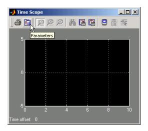
In the **Time Scope parameters** dialog box, set the **Number of axes** parameter to 2 and click **OK**. Now, the **Time Scope** window has two plotting windows and the Time Scope block has two input ports.
