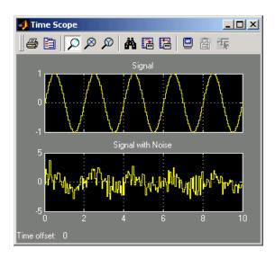
**Note** You can change the signal labels in the **Time Scope** window by right-clicking on the axes and selecting **Axes properties**. In the **Title** text box, enter your signal label.
