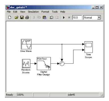
**3** Run your model and view the results in the **Time Scope** window. This window shows the original input signal and the signal with low frequency noise added to it.
